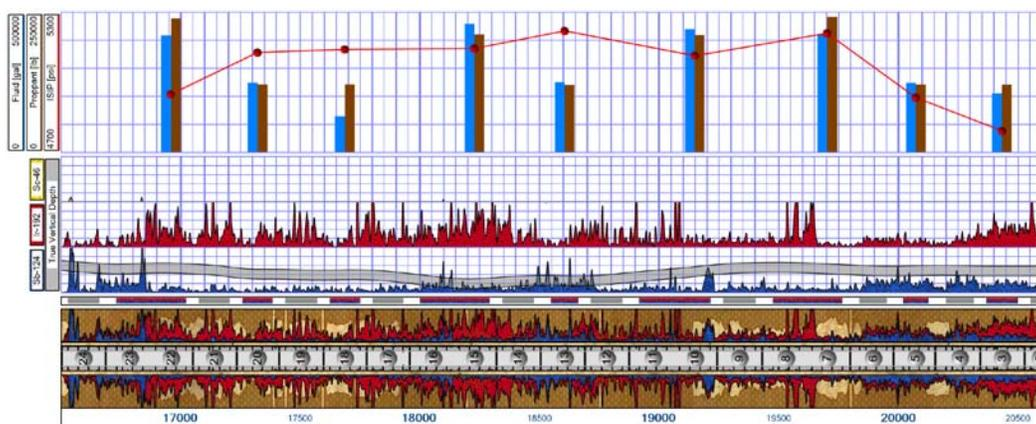
Figure 9—Spectral gamma ray log for TF-1H Well
