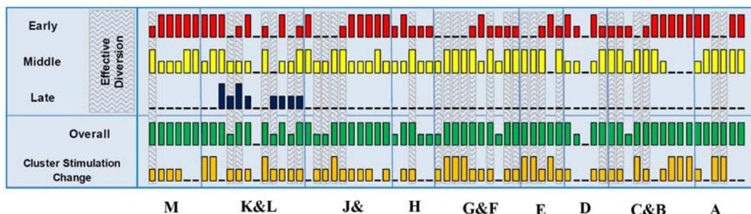
Figure 8—Diversion analysis for well MB-1H
