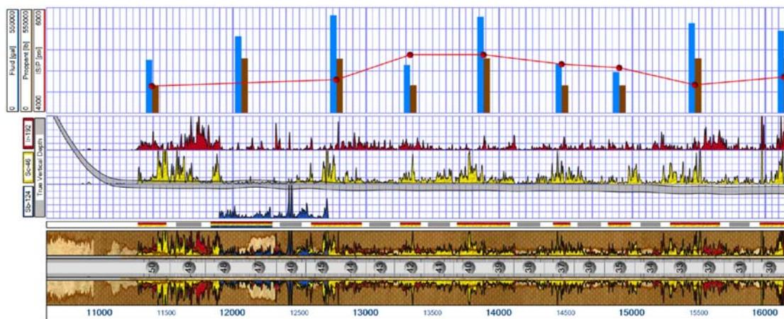
Figure 7—Spectral gamma ray log for MB-1H Well.
